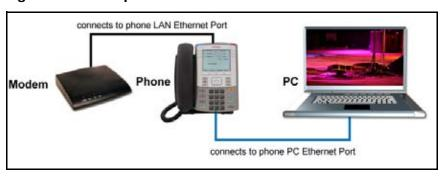
Figure 8: IP Deskphone connected to the router
